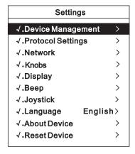
Device Management: Used to manage the keyboard neglect device and added device information; Protocol Settings: Authorization and information management for the corresponding protocol of the controller:
