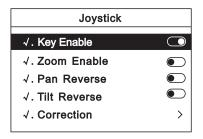
Key Enable: After turning on, click the top button can control the camera back to home position
